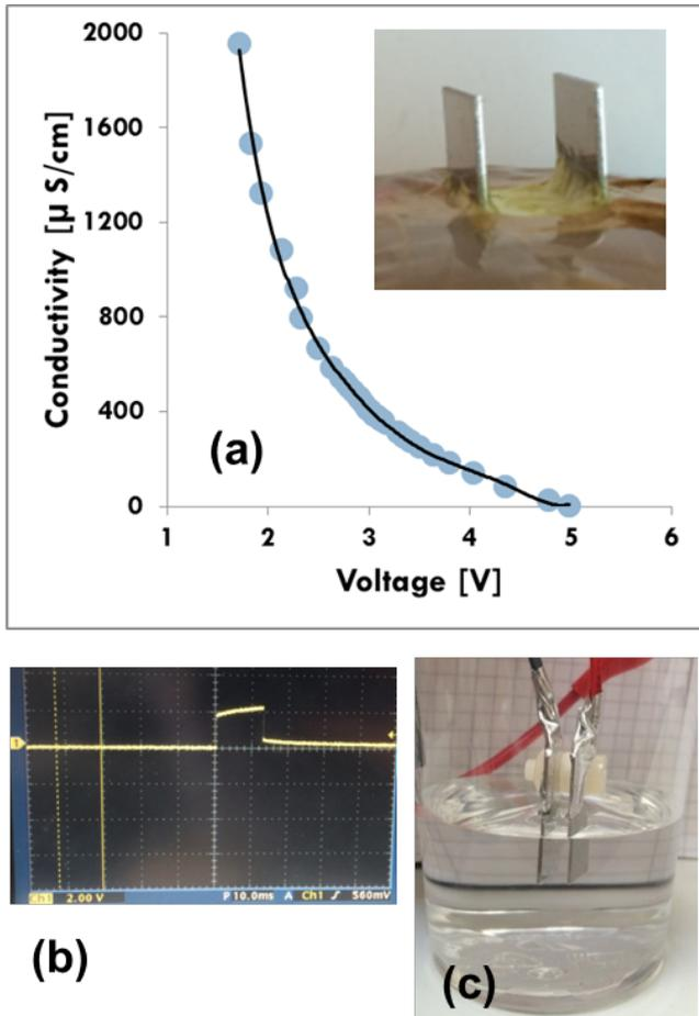
Fig. 3. Conductivity sensing configuration with a) calibration curve (inset: photo of the sensor electrodes), b) the electrical measurement pulse and c) a photo of the experimental setup for the calibration procedure
