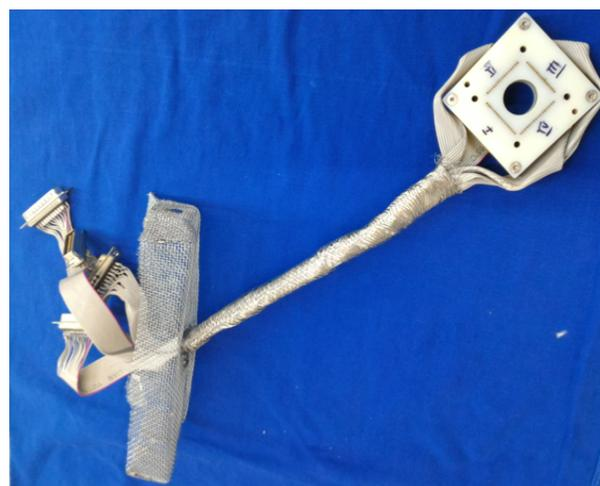
Fig. 3. Supporting apparatus to connect the array and to measure the potentials, and electromagnetic shielding. Source: authors.
